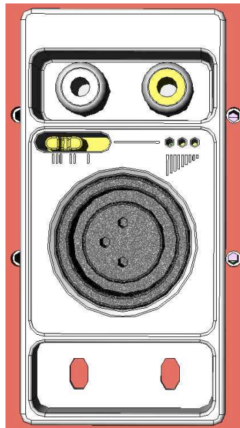
Figure 3-4: Graphic showing AMX0.2CN label recess (bottom of fascia plate) with label screw holes.
