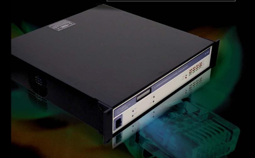
The SI-series amplifiers employ a Class D output topology for maximum efficiency and does not require high volume, forced fan cooling even with the amplifier running into clip on all channels. In addition, the switch mode power supply (SMPS) incorporates power factor correction (PFC) to comply with incoming legislation and minimize noise pollution of the electrical supply.
