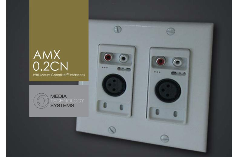
The AMX0.2CN is a 2-gang wall mount CobraNet<sup>®</sup> interface with 2 analog line level outputs, 16 CobraNet<sup>®</sup> input streams and 8 CobraNet<sup>®</sup> output streams. The internal DSP processing provides a 12 channel AutoMixer with signal processing for EQ, High Pass, Low Pass, Compressor and Delay, including remote triggering of camera positioning presets. In addition, 5 AMX0.2CN's can be combined to make a 56x10 matrix.
