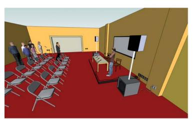
The small meeting room system has two AMX0.2CN's either side of the head table, where the powered loudspeakers are plugged into the AMX0.2CN's. The head table microphones are plugged into ION2.0 wall mount interfaces, as are the boom arm microphones used for taking questions. The ION2.0's stream audio over the network to the AMX0.2CN and all control and configuration is done via a local or remote laptop or PC (see block diagram below).
