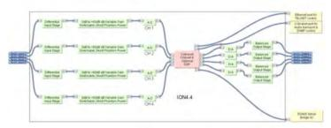
System block diagram (above) of the ION4.4 (ION8.8 is identical, except for 4 more analog inputs and 4 more analog outputs).
