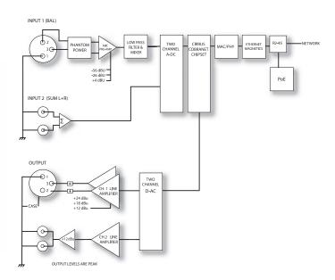
The ION1.1 output section converts 2 channels of incoming CobraNet® data stream back into analog audio signals. Channel 1 is the RCA output, which are -8dBu nominal (+12dBu peak) and a mono output (ie left & right channels have the same signal).
