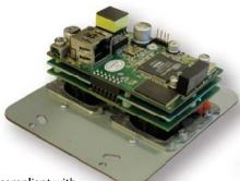
The ION1.1 is fully compliant with the CobraNet® protocol and will connect to any 3rd party Control Room DSP solution. Converting to CobraNet® at the wall reduces problems with buzz, hum, ground loops and other cable issues. In addition, the system design no longer needs special isolation and impedance matching interfaces to connect a customer's laptop via a long analog cable back to the AV switcher in the control room.
